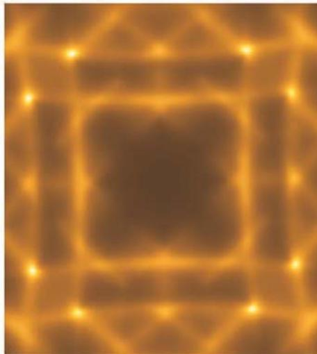
Thermal diffuse scattering (TDS) from Si. The data were collected in a transmission geometry (photon energy 28 keV) using an image plate detector. The data were collected on the UNI-CAT beamline at the Advanced Photon Source in an exposure time of  $\sim 10$  s. The top and bottom left panels show the data taken with a (111) and a (100) axis parallel to the incident beam respectively. The data are plotted on a logarithmic scale.
